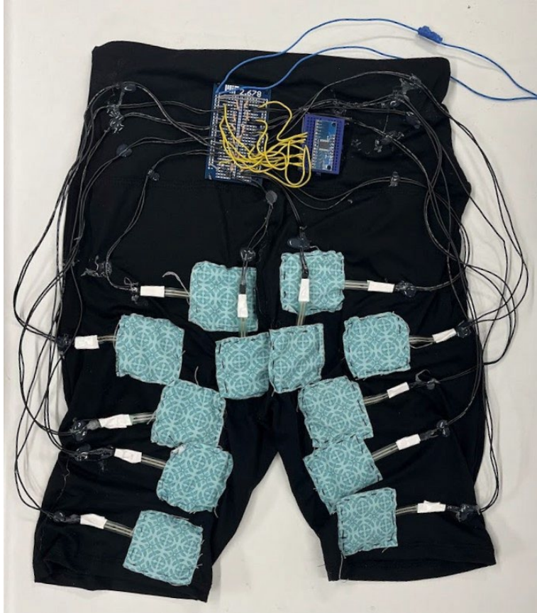
Fig. 10: An image of the prototype, demonstrating the 12 FSR resistor sensor layout as well as the electronics layout.
