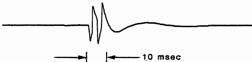
Figure 6.5 - Microphone response to tapping on the case. Since the force on the back of the case compresses the air in the chamber, negative initial deflections in patient data are interpreted as first half cycles of the chest moving toward the microphone. The microphone was placed on the arm for this experiment. The point of interest is the direction of the initial deflection rather than the details of the response.
