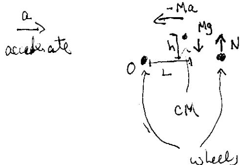
$$\text{torques around } O: h Ma - L Mg + 2LN = 0$$
