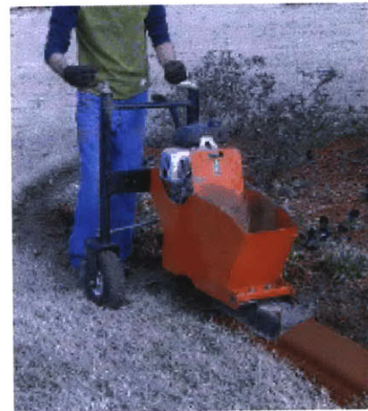
Figure 23. Curving machine is normally used for landscaping or for building curves at side walks
