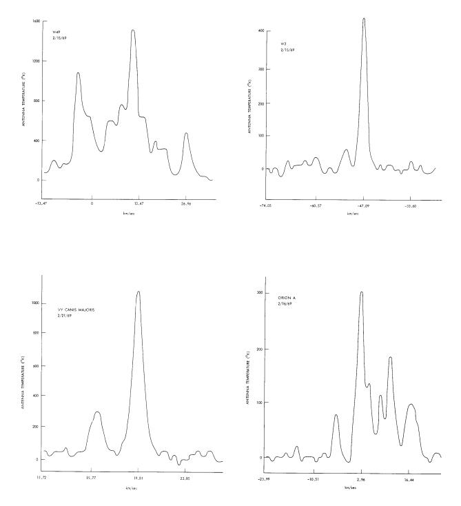
Fig. III-2. Interstellar H<sub>2</sub>O Spectra. Antenna temperatures are uncorrected for atmospheric absorption and velocities are with respect to the local standard of rest.
