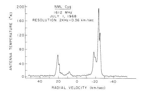
Fig. III-1. The 1612-MHz spectrum of the infrared (IR) star NML Cygni. Antenna polarization was left circular, and integration time was 12 min.
