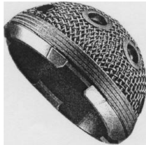
Fig. 2. The metal mesh on this acetabular cup is to serve at the bone attachment vehicle. Bone tissue ingrowth into the metal mesh will allow fixation to be achieved. The polyethylene insert is not shown.
