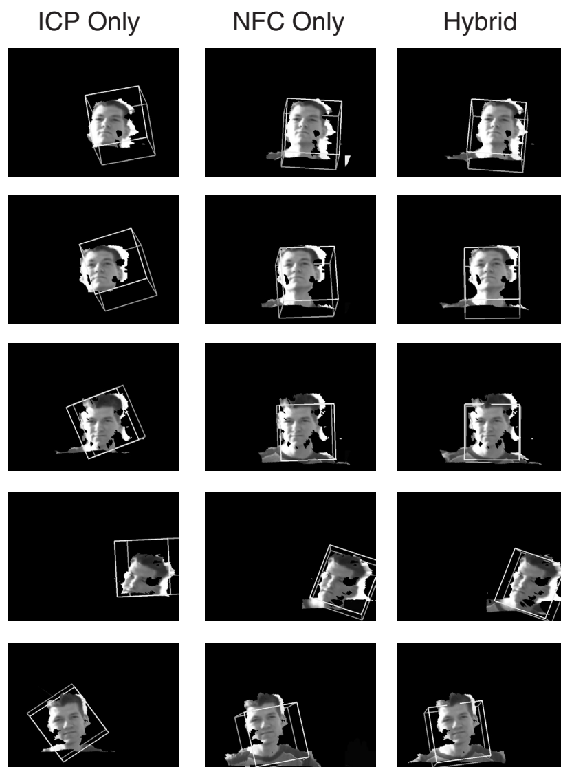
Figure 5.8: Face tracking results for sequence 3. Each row represents tracking results at different frames: 135, 150, 170, 195, and 250.
