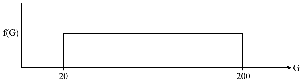
Figure 1. Probability density function for wind-powered plant output, G = Units of MWe.
