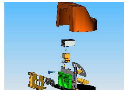
The beta prototype was actually taken to Mali. “The crew discovered the water jet cutter. Entire device is composed of plastic sheets machined in the cutter.” Since the film plane is horizontal, the optical path is more direct leading to fewer parts, lower cost. Note the small fan at the bottom, forcing air across the pin based heat sink.; it turns out the power consumed by the fan more than paid off in terms of improved LED performance and reliability.
