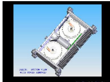
Exploded view. Notice all the screws; you couldn't achieve \$50 system cost target with so many individual pieces, instead do it with snap fit. There's a small microprocessor on board to manage the 12V to 6.5V switching power supply and current regulator, also monitors temperature (auto shut-down) and logs lifecycle data via software.
