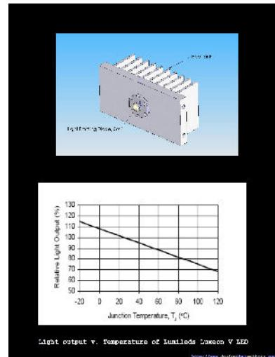
Schematic of the 3<sup>rd</sup> generation (gamma) prototype design. The device gets smaller and simpler. The heat sink is integrated into the package itself – an extruded aluminum piece. It turned out that funding decisions were delayed; the extrusion die was too expensive for a small run (10 units), so Alan made a single version on the lab’s CNC lathe by hand.
