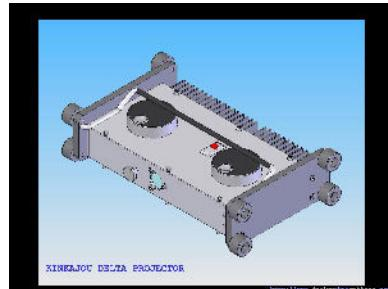
Delta bottom view with cover removed. Focus happens by sliding the knob by the lens in or out of the box. Frictional drag and a 1-way clutch on each reel keeps the film in place, allows it to forward appropriately.
