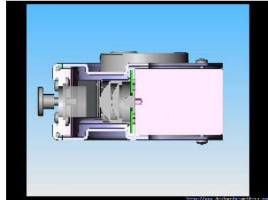
4<sup>th</sup> generation (delta) schematic. Very similar "guts" but the box is simpler, lower costs, using off the shelf heat sink rather than a custom die.
