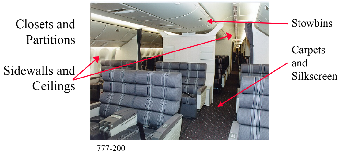
Figure 3 A representative picture of the some of the commodities the Interiors Responsibility Center provides the 777 factory. Pictured above is the 777 –200.
