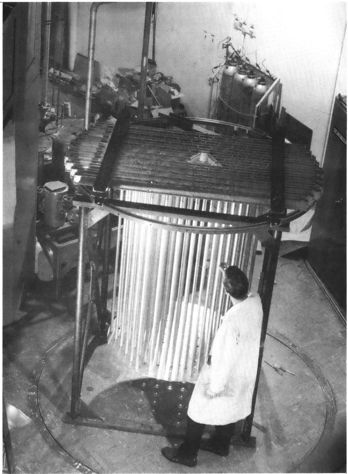
FIG. 6.3 4\frac{1}{2} INCH SPACING LATTICE BEFORE INSERTION INTO TANK
